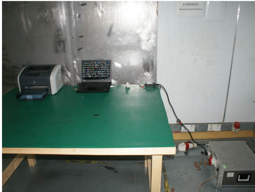
Photograph 6: Set-up for Radiated Emissions, below 1GHz
