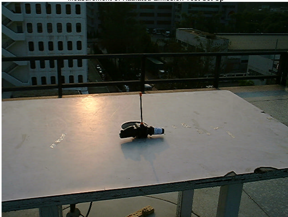
Measurement of Radiated Emission Test Set Up
