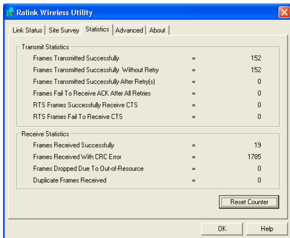
Use this feature to see how many packets have been successfully transmitted and received on your network. The **Reset Counter** button allows you to set all counters back to zero.
