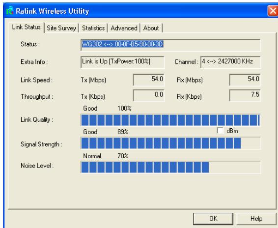
**Status** - Displays the BSSID (Basic Service Set ID) of the access point to which the Wireless LAN USB adapter is associated. The BSSID is the 6-byte hexadecimal ID number (the MAC address) of the associated access point or base station. This information is only displayed, and not configurable. Clients that have been associated with the same access point, will display the same BSSID.
