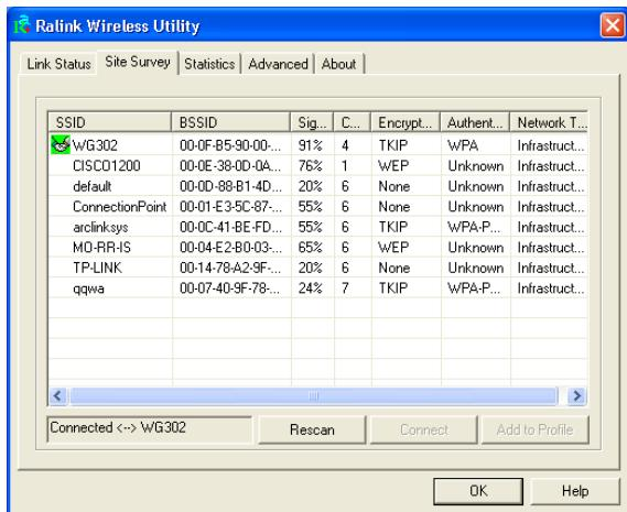
**SSID** - Service Set ID. The SSID is a code attached to all packets on a wireless network to identify each packet as part of that network. It is essentially the name of your network and can be up to a maximum of 32 alphanumeric characters in length. The green icon beside SSID WG302 shows you are connected to this network.
