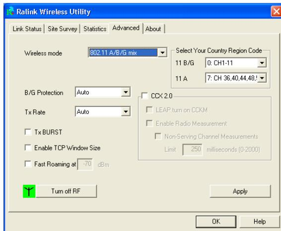
**Wireless mode** - The RALINK Wireless Network Card supports 802.11a, 802.11b and 802.11g mode. (Default: 802.11 A/B/G mix)
