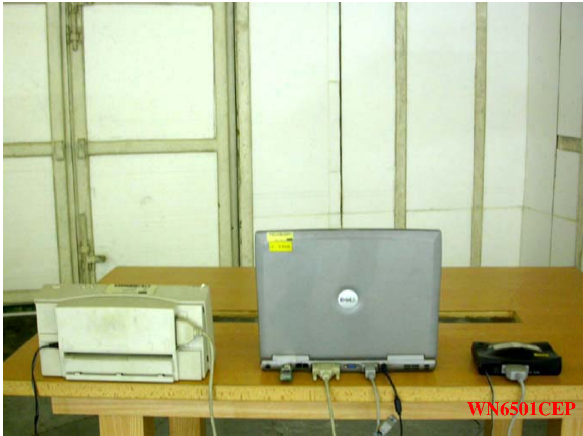
Photo 3: Radiated Emission Test Set-up
