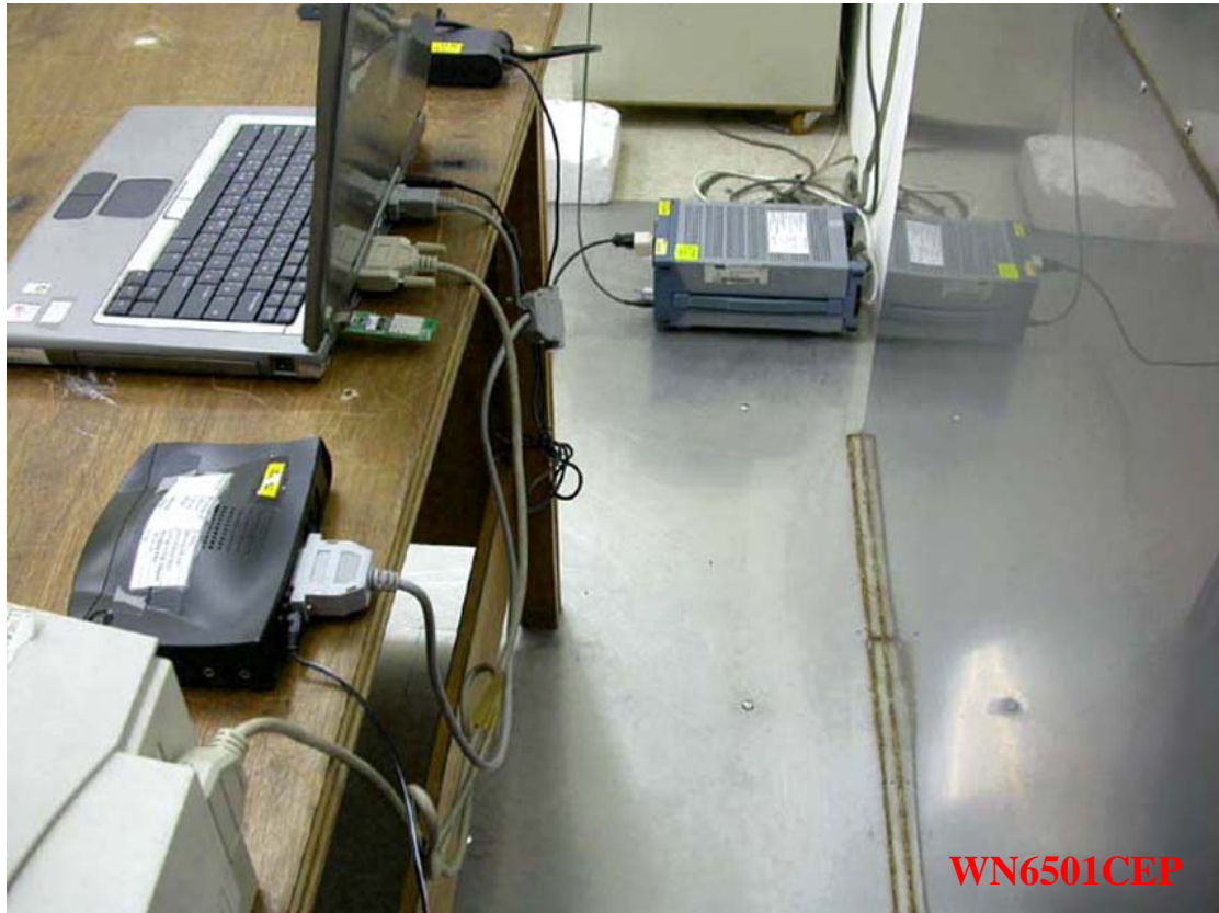
Photo 2: Conducted Emission Test Set-up
