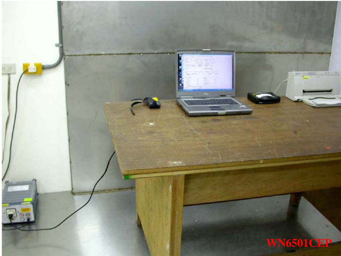
Photo 1: Conducted Emission Test Set-up
