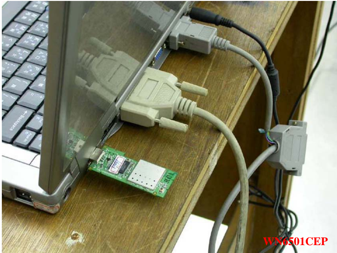
Photo 3: Conducted Emission Test Set-up
