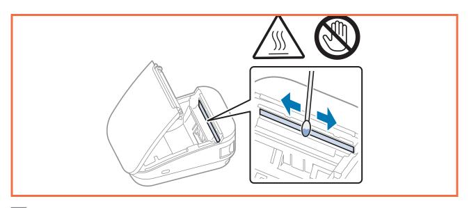
When the cleaned area is completely dry, load the roll paper and close the roll paper cover.
