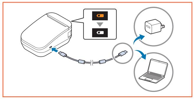
Disconnect the USB cable from the printer.
