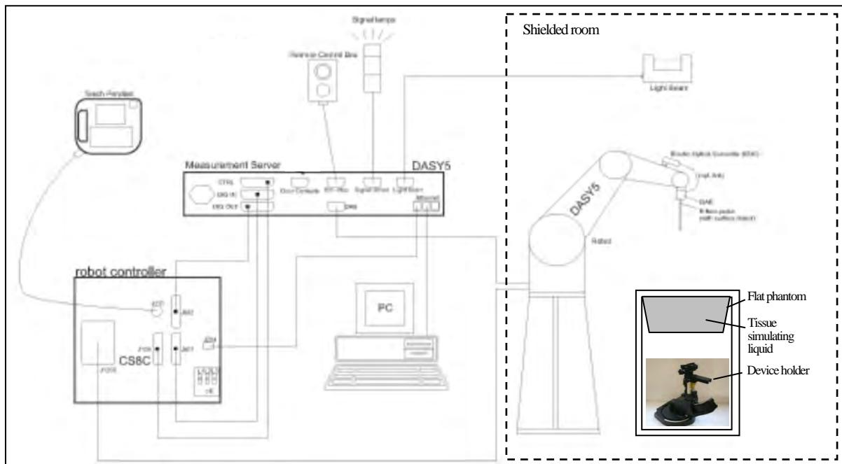
The DASY5 system for performing compliance tests consist of the following items:
