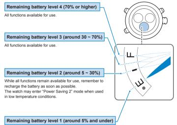
Some functions are unavailable for use. Please recharge the watch. At level 1 the following constraints are placed on the movement of the short seconds hand (seen in the diagram below).
