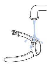
If charging or communicating becomes unstable, clean the contact points on the device and the cradle with a damp cotton swab.
