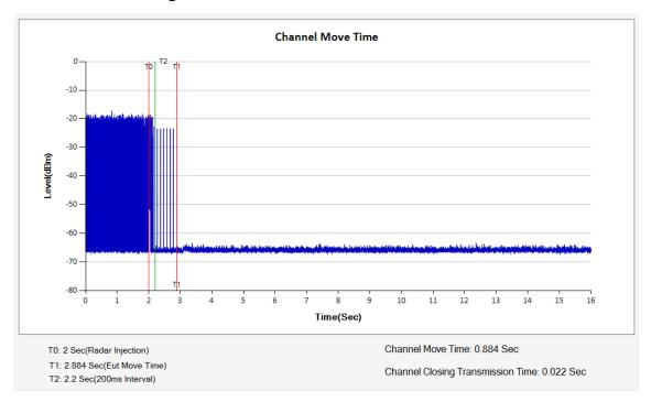
Verdict: Note: narrowing the sweep time as the good engineering process for the verification of transmission closing in 200ms
