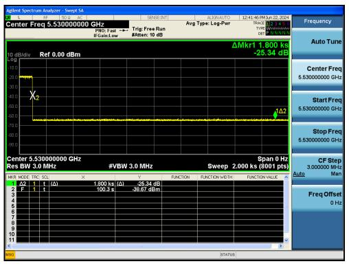
Verdict: To verify whether channel is unavailable to be operated in 30 minutes. 1.8ks = 1800s = 1800 s/min /60 = 30minute
