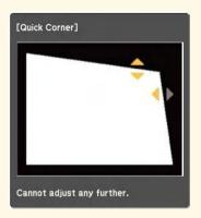
To reset the Quick Corner corrections, hold down [Esc] for about 2 seconds while the Quick Corner adjustment screen is displayed, and select Reset Quick Corner. Select Switch to H/V-Keystone to switch the image shape correction method to H/V-Keystone.
