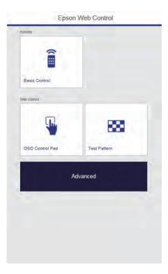
To control projection remotely, select **Basic Control**.
