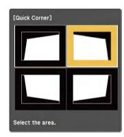
Press the arrow buttons to adjust the image shape as necessary.
