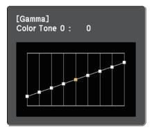
• To use the gamma adjustment graph, select **Adjust it from the graph**. Press the left or right arrow buttons to select the color tone
