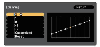
When you select a smaller value, you can reduce the overall brightness of the image to make the image sharper. When you select a larger value,
