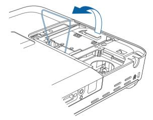
6 Lift up the lamp handle and carefully pull the lamp out of the projector.
