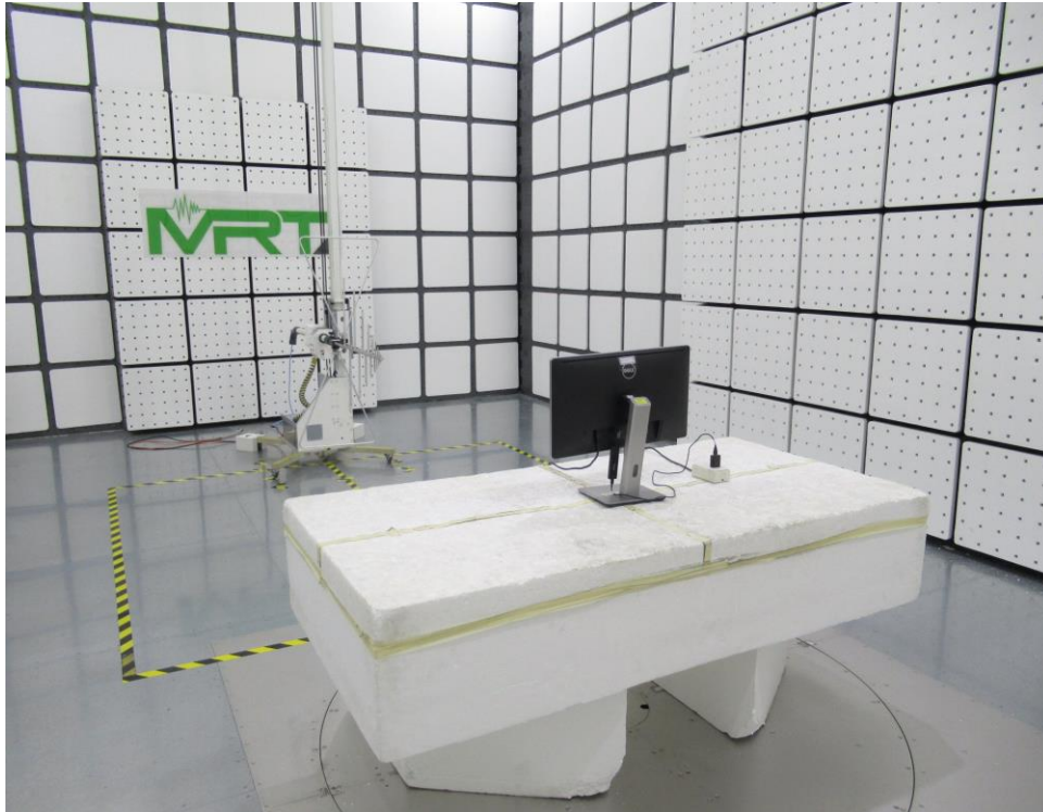
Description: Radiated Spurious Emission Test Setup for Above 1GHz
