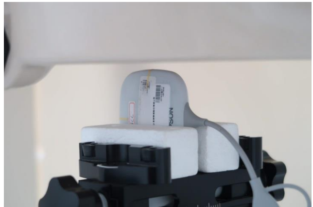
Vertical Front, Test Separation 5 mm
