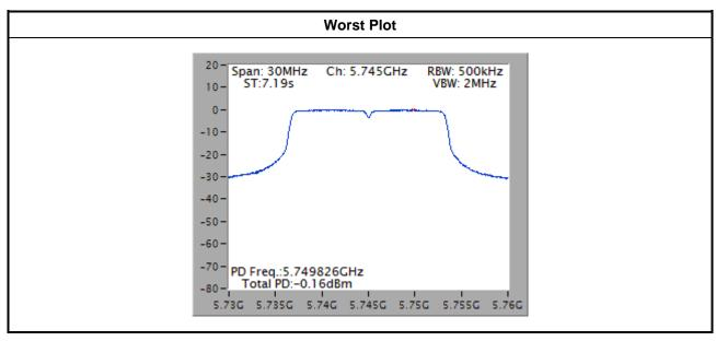
Note: Power Spectral Density plot is without duty factor.
