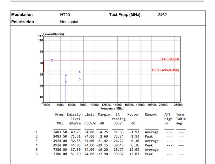
Note 1: Emission Level (dBuV/m) = SA Reading (dBuV/m) + Factor\* (dB) \*Factor includes antenna factor, cable loss and amplifier gain
