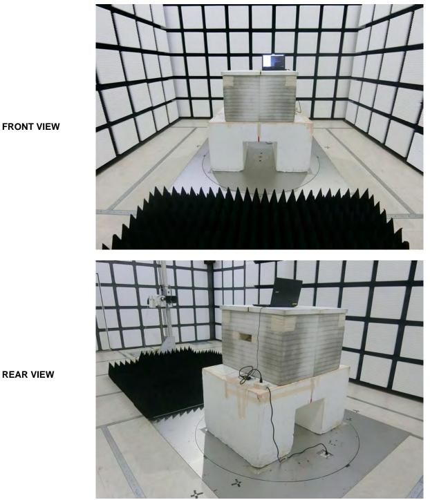
Test Configuration: Above 1GHz / Test Mode: Mode 1~Mode 2
