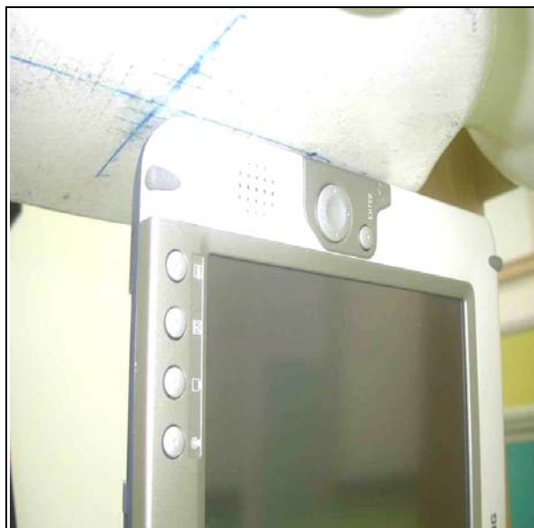
The lateral of the EUT face to the phantom with 0mm-separation distance.
