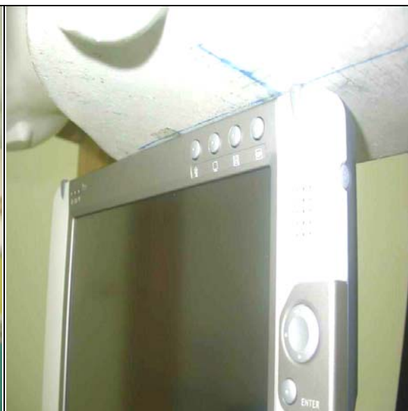
The tip of the EUT face to the phantom with 0mm-separation distance.
