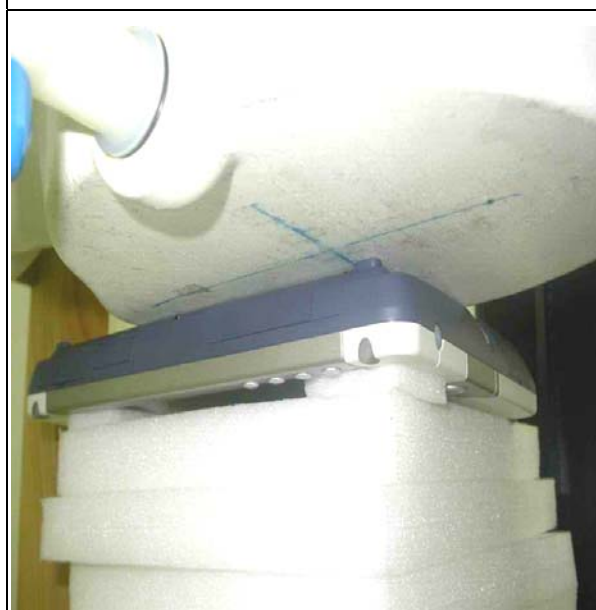
The bottom of the EUT face to the phantom with 0mm-separation distance.
