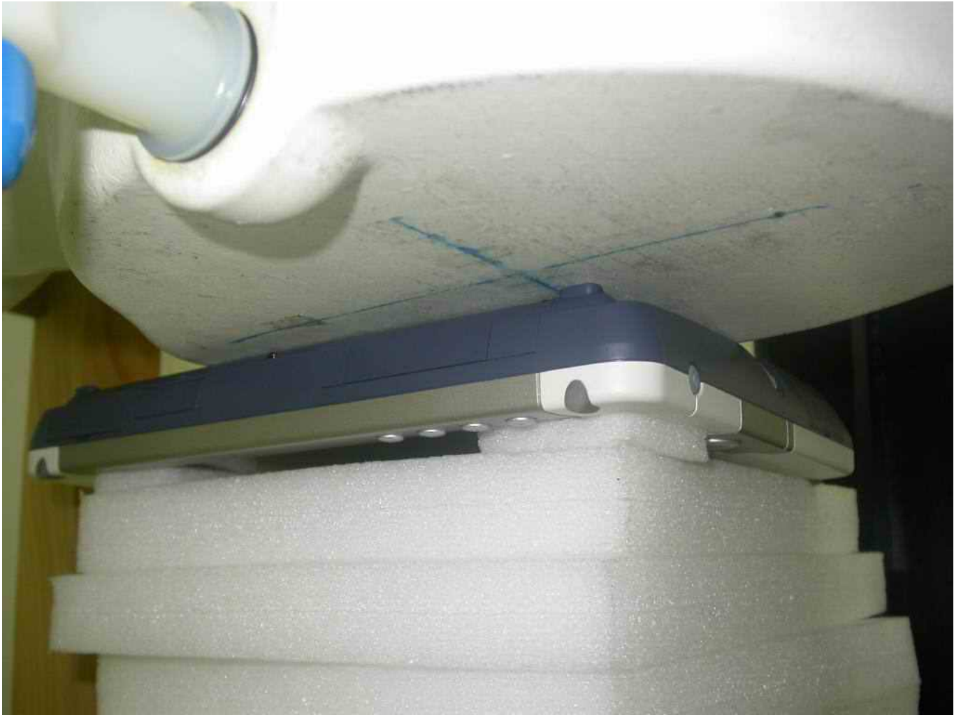
The bottom of the EUT to the flat phantom distance 0 mm EUT Photo
