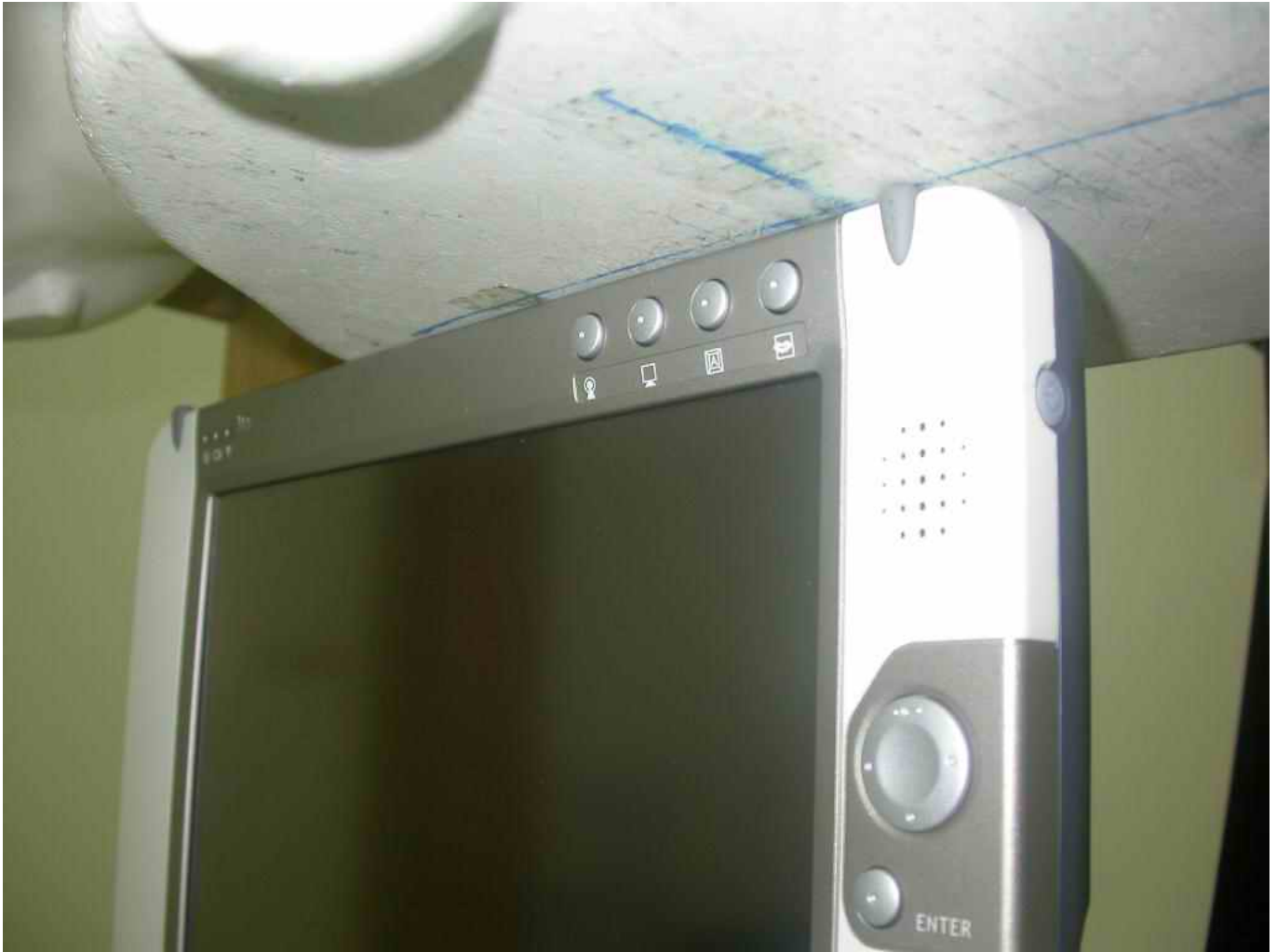
The tip of the EUT to the flat phantom distance 0 mm
