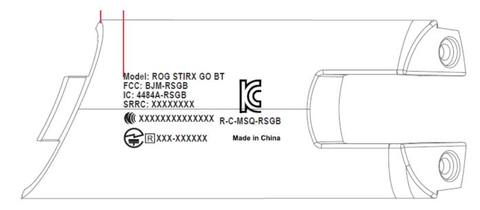
The FCC ID will be placed on the equipment as shown in the photograph below.
