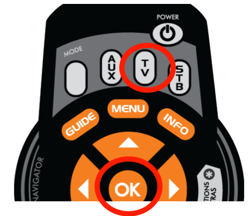
Remote Figure 3: Press the device and OK buttons
