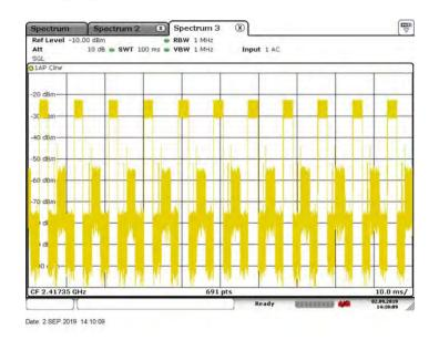
Time on of 100ms= 2.5507ms\*11= 28.058ms Duty Cycle=28.058ms / 100ms= 0.28058 Duty Cycle correction factor= 20 LOG 0.28058= -11.039 dB
