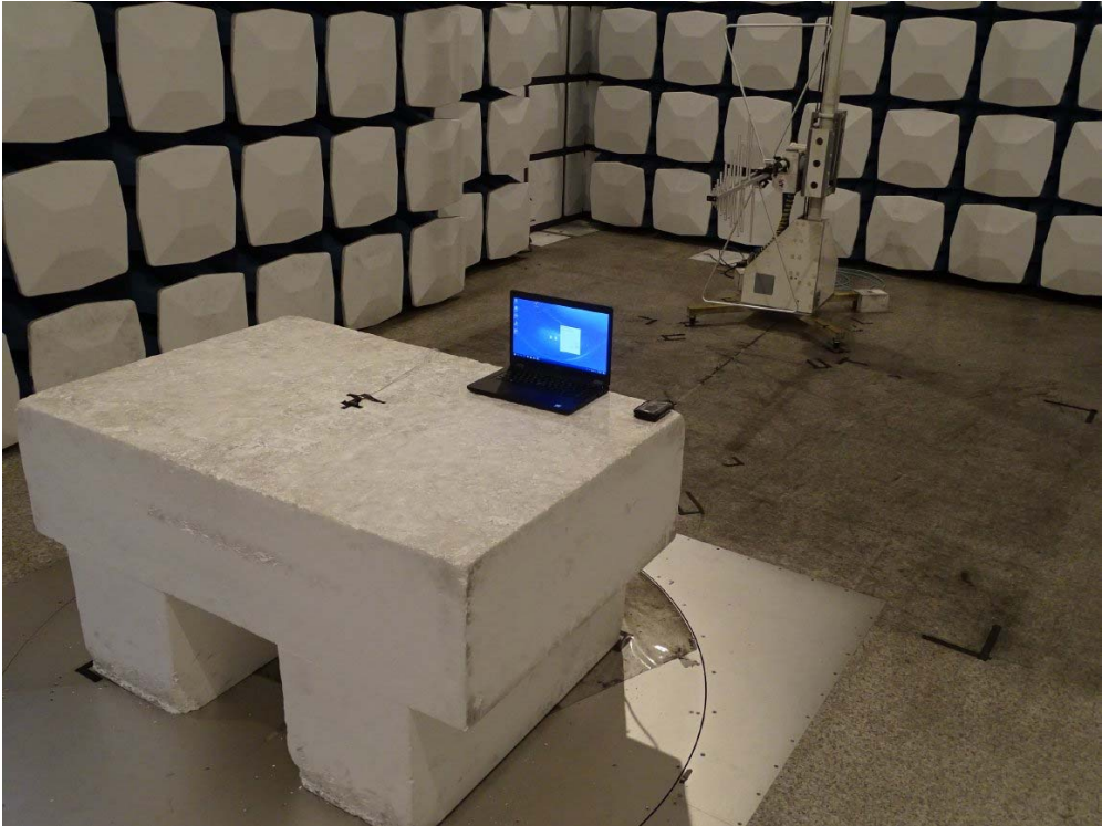
Front View of Radiated Test
