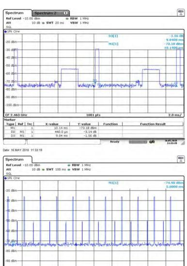
Note: The signals which are under -50dBm are transmitted by the ancillaries.
