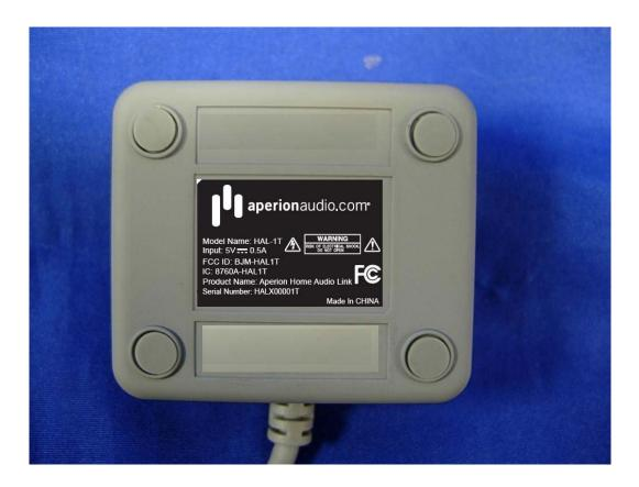
The FCC ID and DocC will be placed on the equipment as shown in the photograph below.
