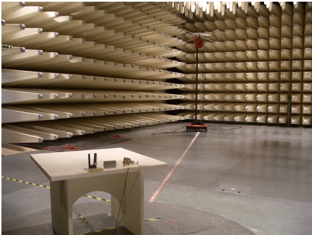
Spurious emission measurement from 30 MHz – 1 GHz. 10 m measurement distance.
