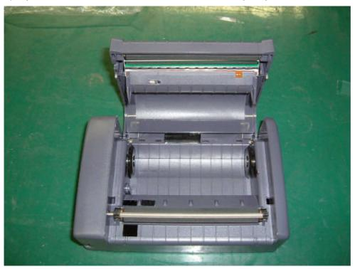
2) With a small tool, such as a pin punch or a jewellers screwdriver, push to release the left and right hooks that secure the head cover to the media cover.
