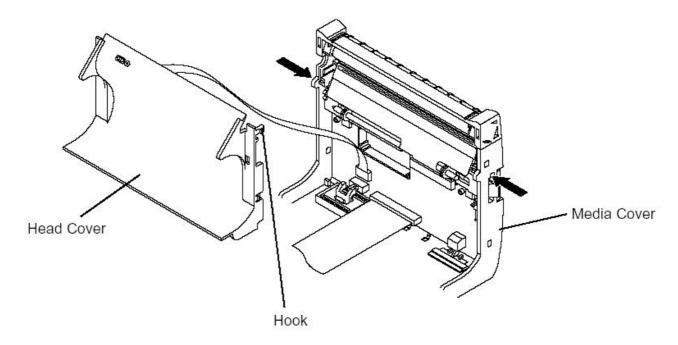
3) Take off sensor PCB with small ribbon cable (sensor FPC) from head cover.
