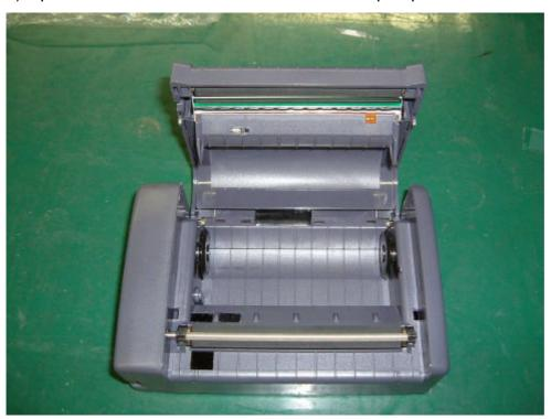
2) With a small tool, such as a pin punch or a jewellers screwdriver, push to release the left and right hooks that secure the head cover to the media cover.
