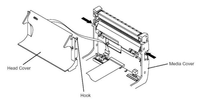
3) Take off sensor PCB with small ribbon cable (sensor FPC) from head cover.
