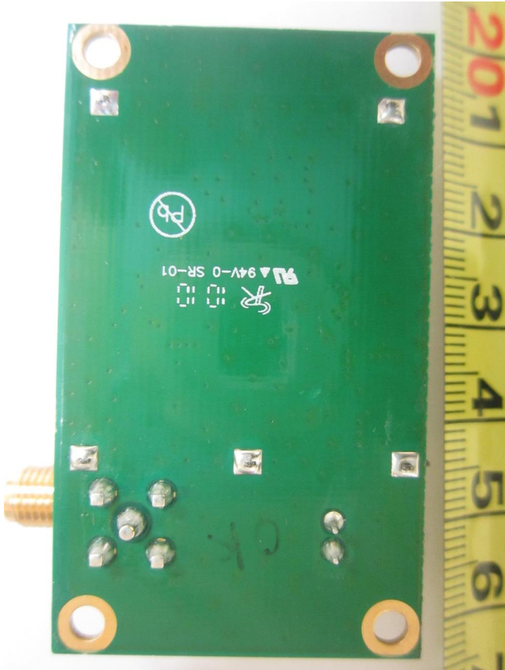
Crystal Board PCB Trace Side
