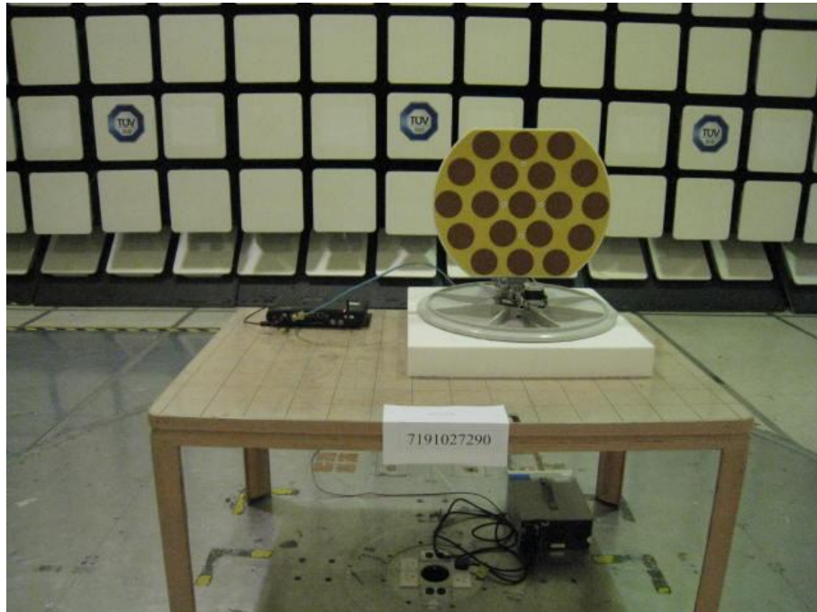
Protection of Aeronautical Radio Navigation Satellite Service Test Setup (Front View)
