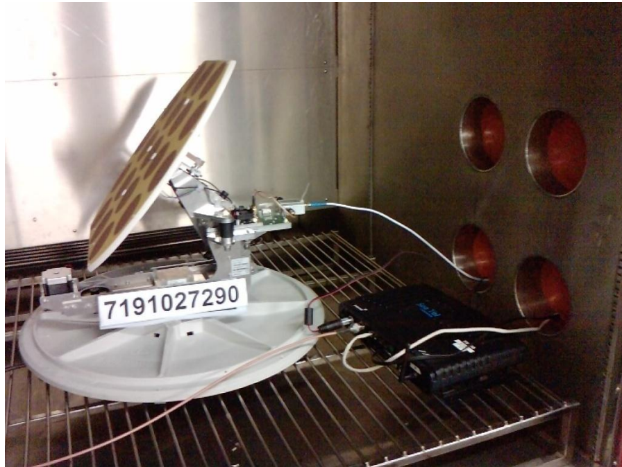
Frequency Stability (Voltage Variation) Test Setup
