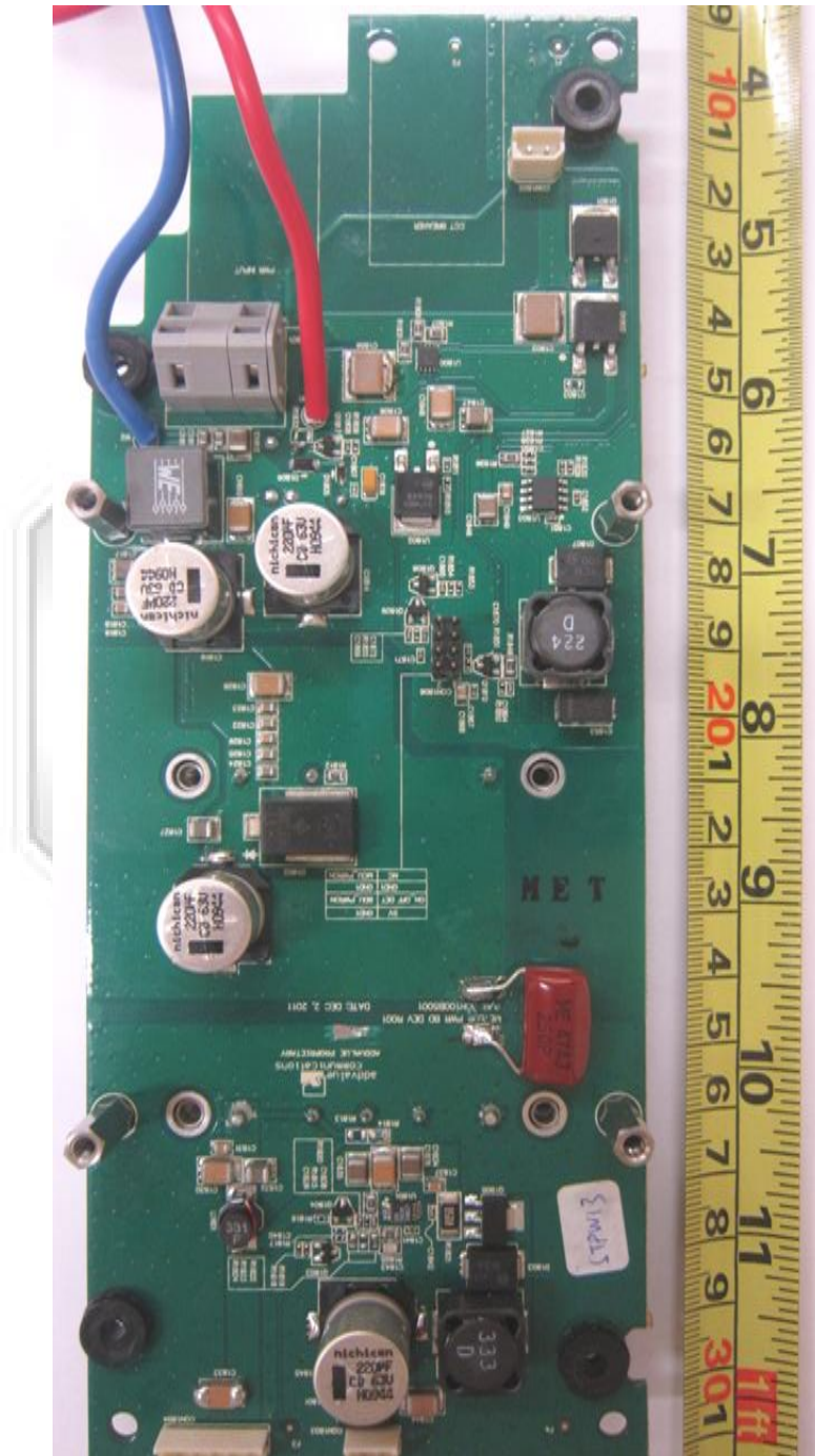
Power Supply PCB Component Side
