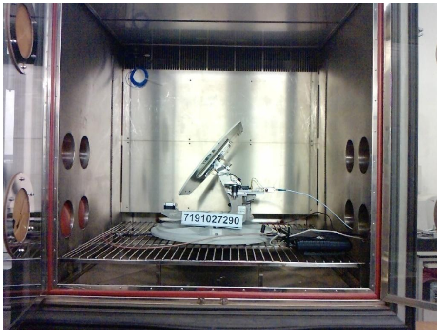
Frequency Stability (Temperature Variation) Test Setup
