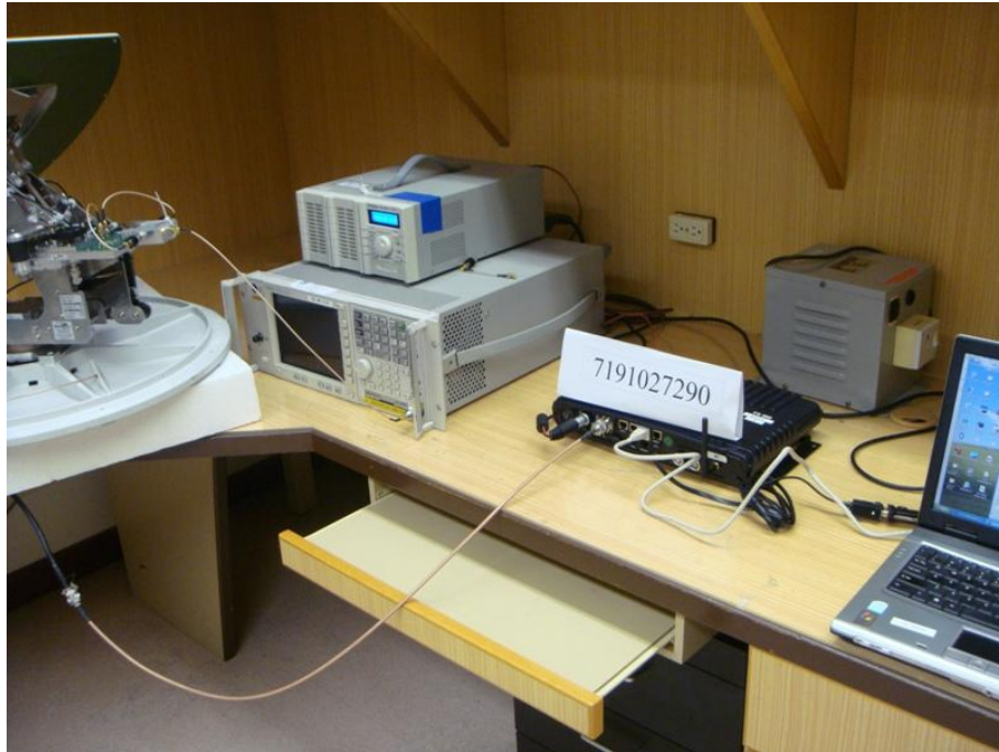
Unwanted Emissions at Antenna Terminal Test Setup
