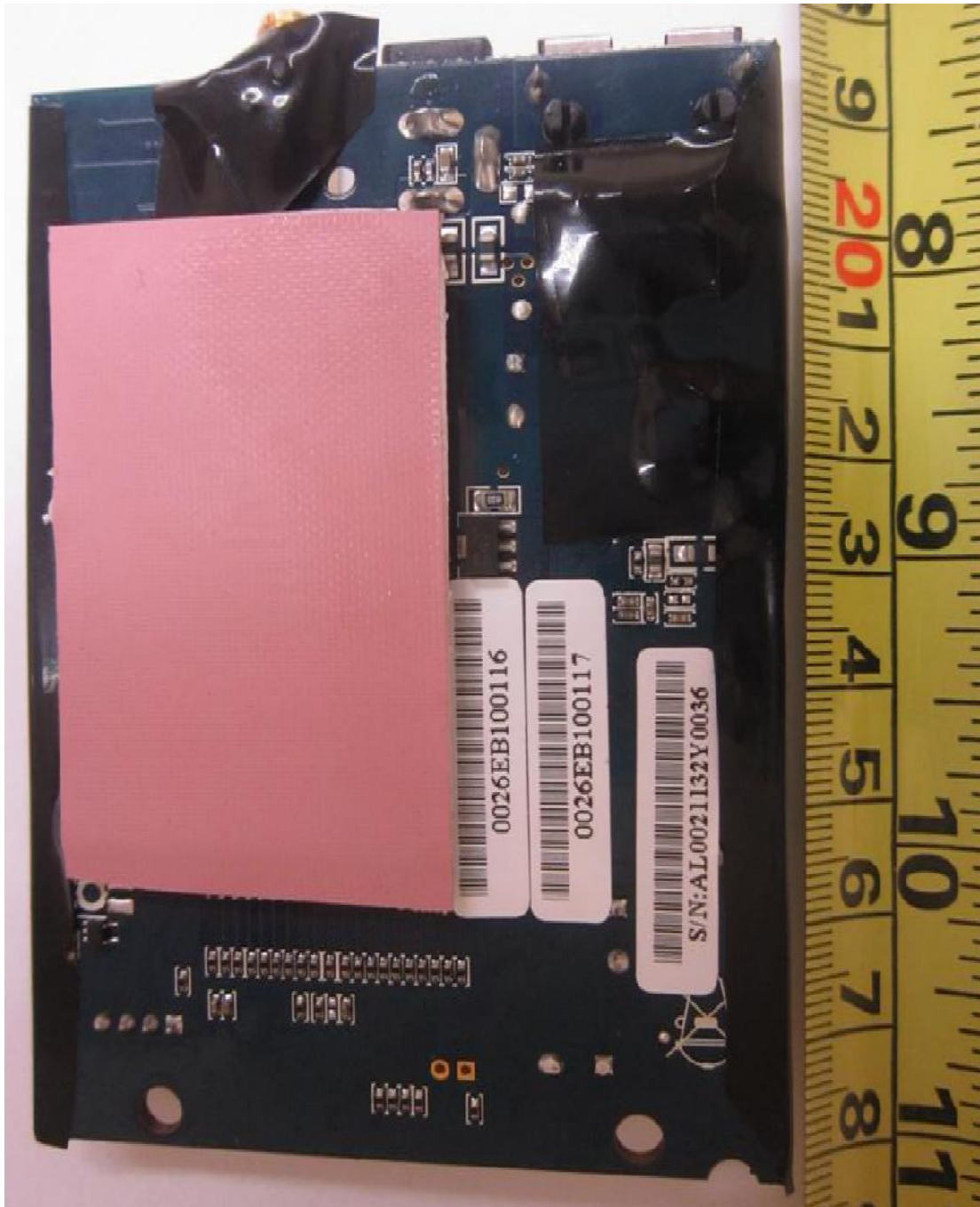
WiFi Module PCB Trace Side
