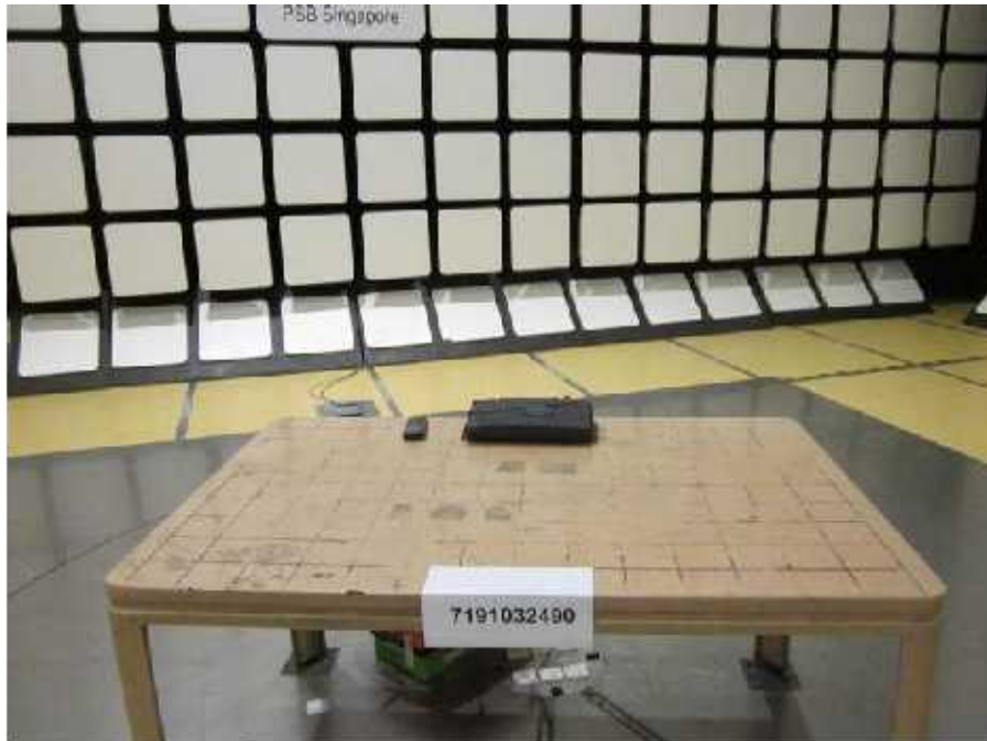
Radiated Emissions Test Setup (Front View)
