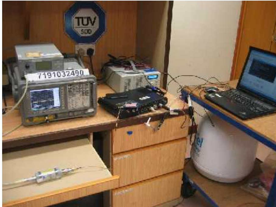
Maximum Peak Power Test Setup
