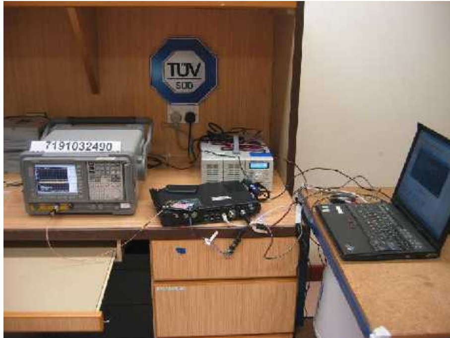
Spectrum Bandwidth (6dB Bandwidth Measurement) Test Setup
