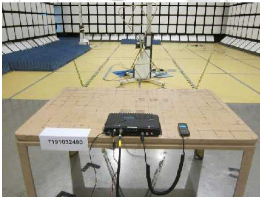
Radiated Emissions Test Setup (Rear View)
