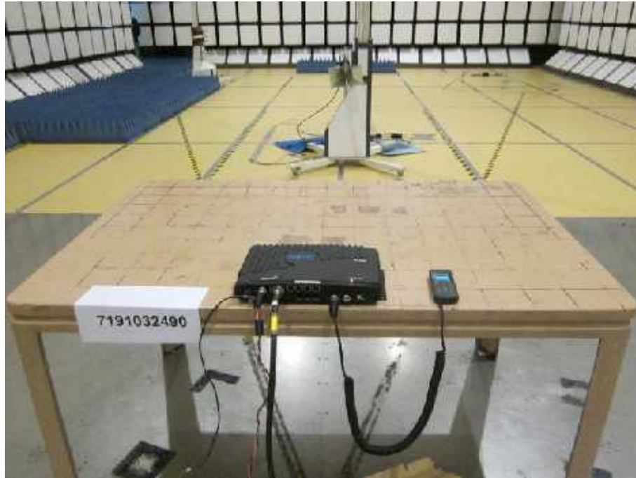
Band Edge Compliance (Radiated) Test Setup
