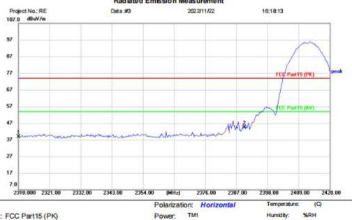
Limit: FCC Part15 (PK) EUT: Wireless Doorbell M/N: WLTRX-3015 Mode: TX-L
