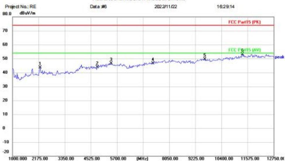
Site Polarization: **Vertical** Temperature: (C)
