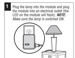
If the lamp is not ON, press and release the Power button on the module to turn the lamp ON.
