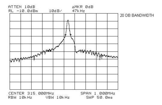
EQUIPMENT: WB-SAW-TX, Wireless Remote Doorbell Transmitter FCC ID: BJ4-62WDB93TX
