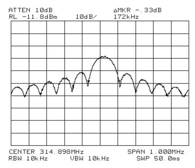
9R02231 W-32A-TX OCC. BW. 20DB 32.768KHZ MODULATION
