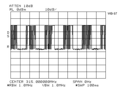
5 Complete Bursts In 100 ms 13 Bits Per Burst 0.6 ms Maximum On Time Per Bit.
