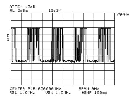
4 Complete Bursts In 100 ms 13 Bits Per Burst 0.6 ms Maximum On Time Per Bit.
