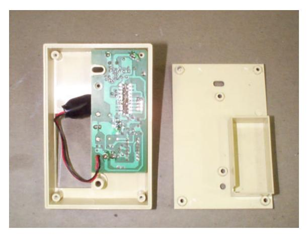
The 6133 Transmitter, when activated by its momentary switch, transmits a modulated code. Setting the jumpers inside the transmitting device configures this code. When a receiving device, programmed via jumpers to the same code as the transmitter, receives this code it then toggles its output state on or off.
