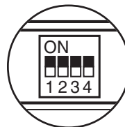
Dip Switches - Shown in the OFF Position (Factory Default)
