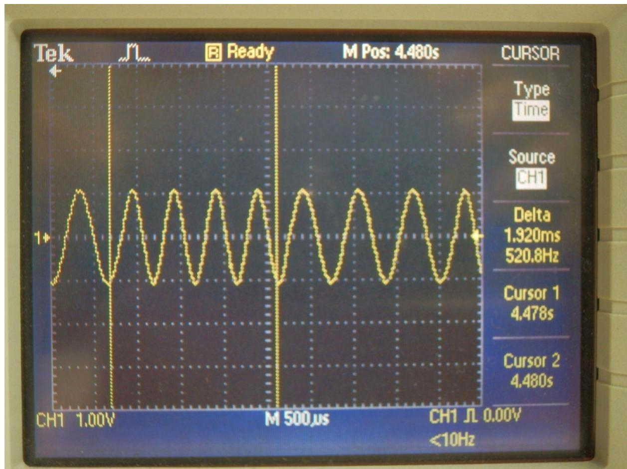
Mark Frequency 2083.2Hz (520.8Hz/cycle x4=2083.2Hz)
