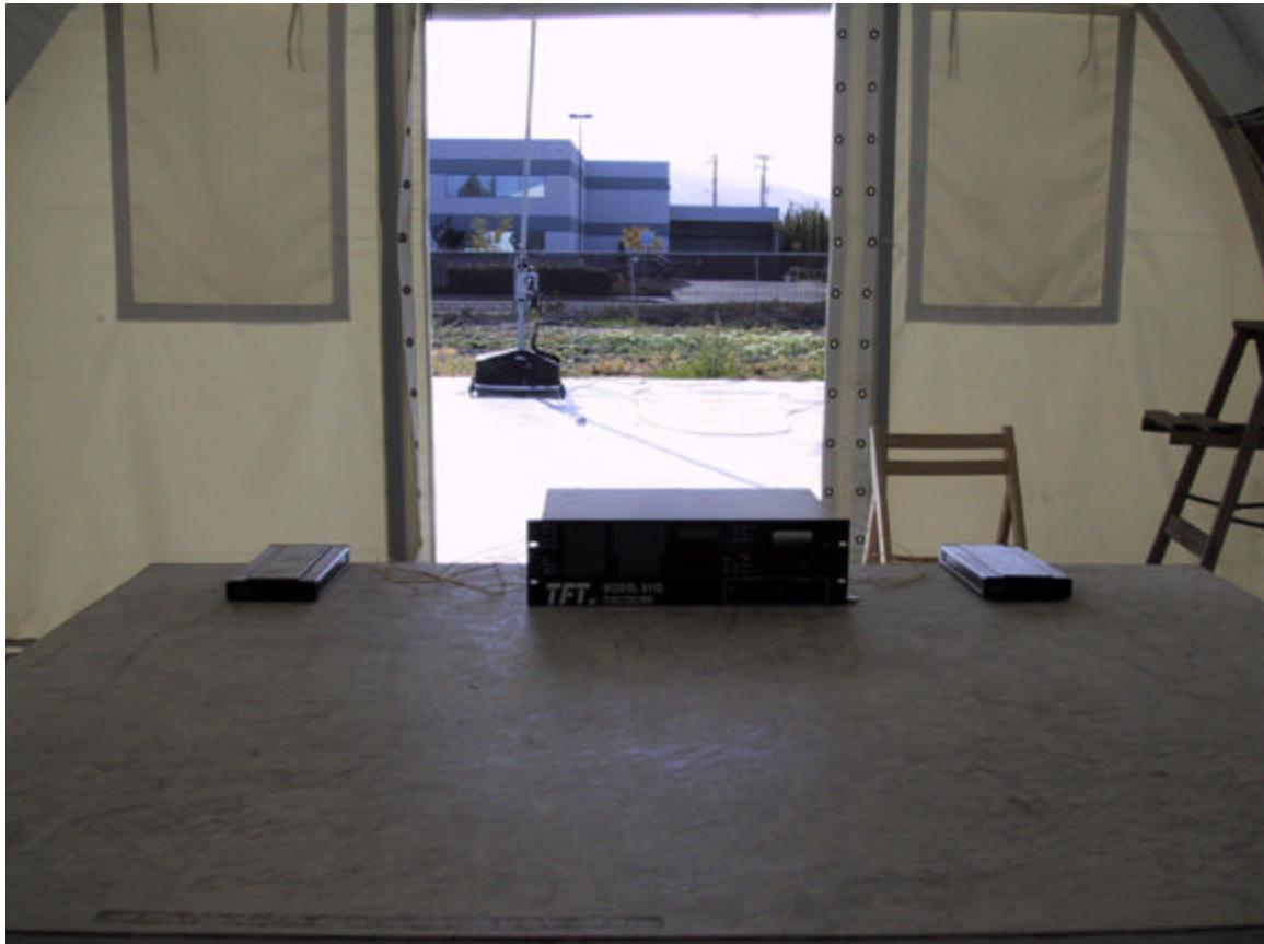
**Photograph 1. Radiated Emissions Test Setup (Front View)**
