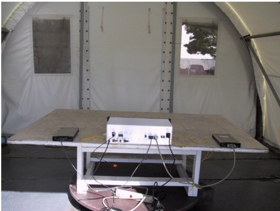
**Radiated Emissions Test Setup (Rear View)**
