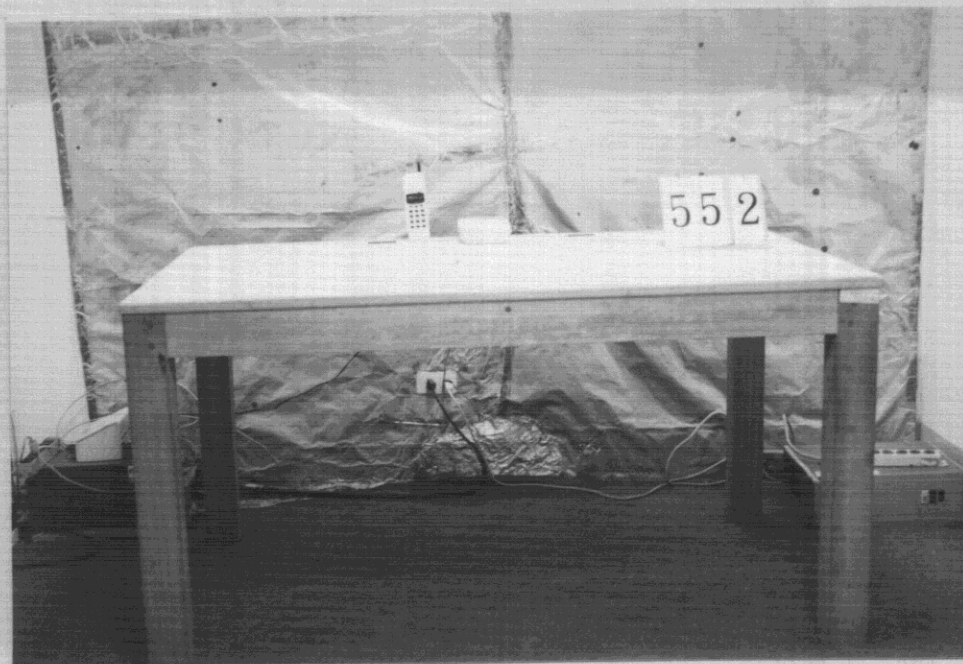
Fig. 4 Conducted emissions test placement (operating only)
