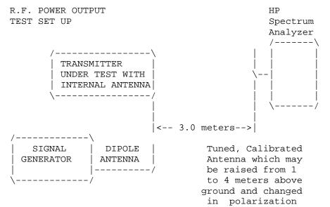
Equipment placed 1 meter above ground on a rotatable platform.
