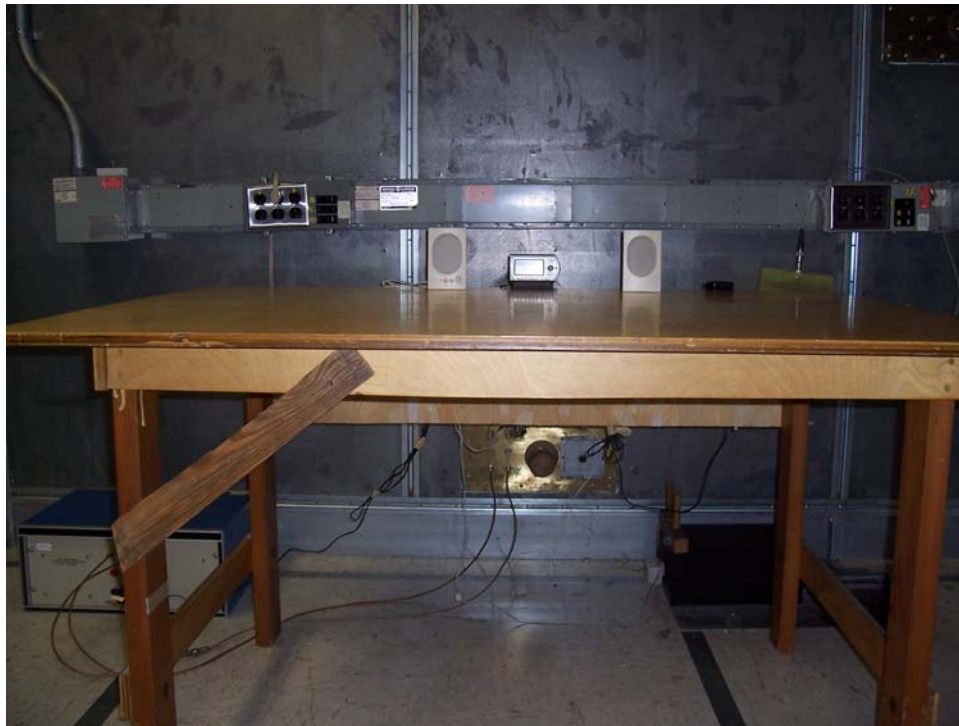
Conducted Emissions Test Setup, View 1
