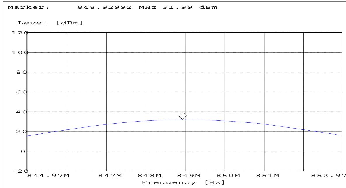
**Field Strength of Spurious Radiation****Subclause §22.917(e)****Measurement Procedure:**
