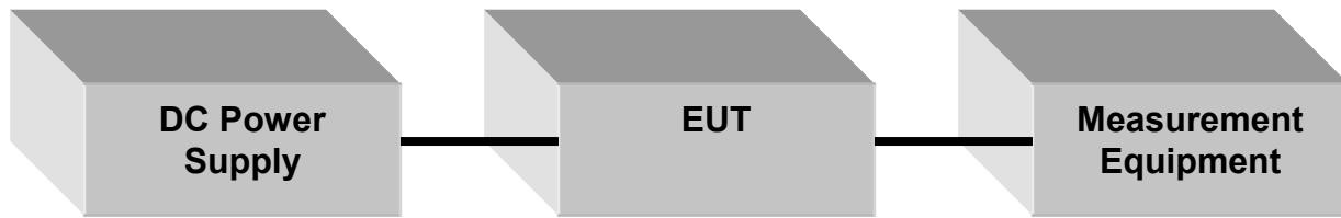
The EUT's RF port is connected to either a spectrum analyser or a power meter with attenuators and co-axial cable.
