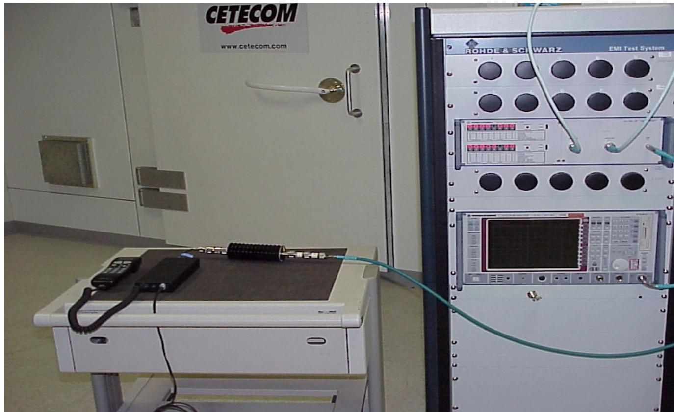
**594N model radiated set-up:**
