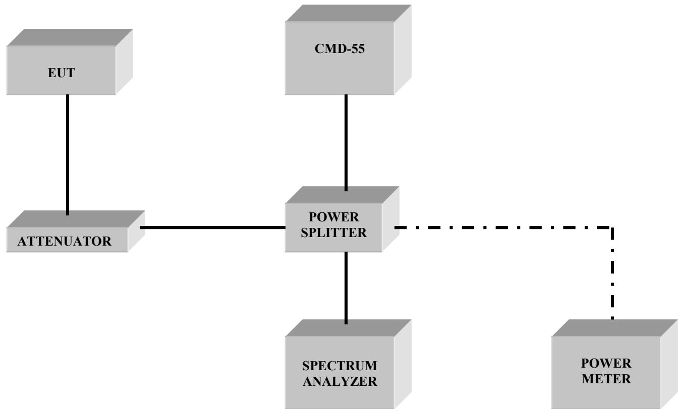
**BLOCK DIAGRAM – Radiated Measurements**
