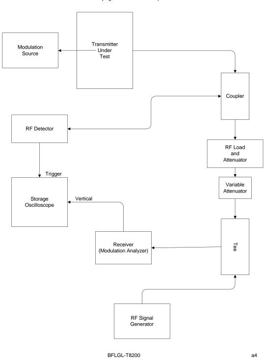
Oscillator Line Voltage Sability Test Setup
