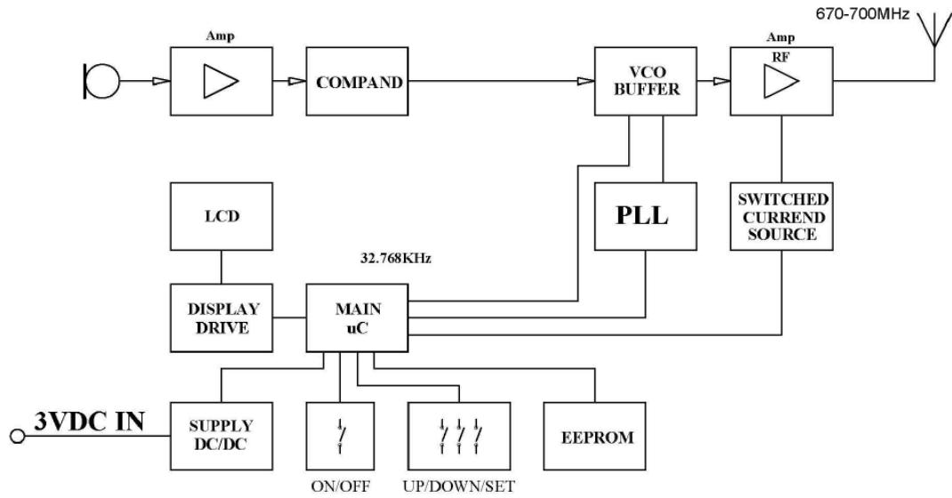
The MIC has transformed the collect voice to digital signal and input it to the audio amplifier, the audio amplifier magnified the signal and after the companding to modulate with the carried frequency by the VCO which was controlled by PLL. The modulated high frequency passed the frequency amplifier to amplify the power and pass the BPF to the high frequency ANT. The DC power supplied by 2\*AA battery, and input to MCU, The channel frequency was changed by PLL which was controlled by MCU.
