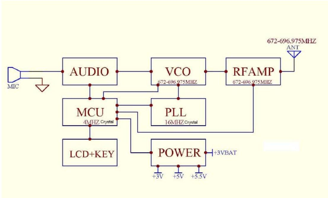
The MIC has transformed the collect voice to digital signal and input it to the audio amplifier, the audio amplifier magnified the signal and after the companding to modulate with the carried frequency by the VCO which was controlled by PLL. The modulated high frequency passed the frequency amplifier to amplify the power and pass the BPF to the high frequency ANT. The DC power supplied by 2\*AA battery, and input to MCU, The channel frequency was changed by PLL which was controlled by MCU.
